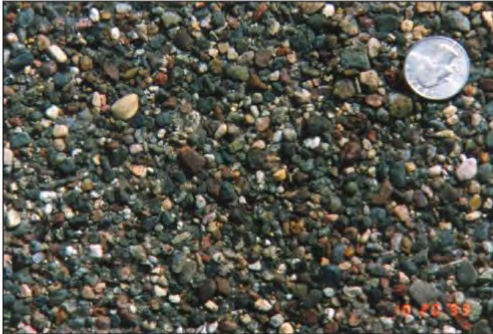
Figure 1.1. Example of an FA-2 Pea Rock (buckshot)
