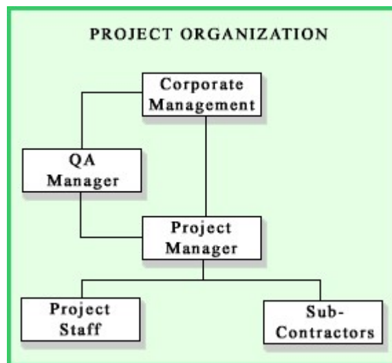
Figure 3 - A possible organization structure showing the principal QA position on a project.
