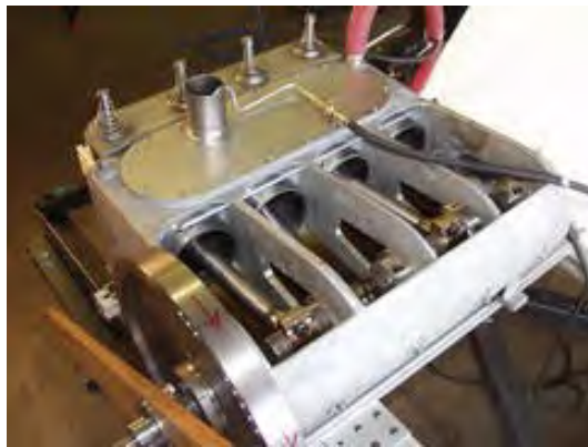
Figure 2: Assembled replica engine of Wright Brothers first plane with sheet metal side cover of crankcase removed to show novel Aluminum engine block/crankcase construction with iron cylinder liners. Major components of the original engine were donated to various museums and never returned.
