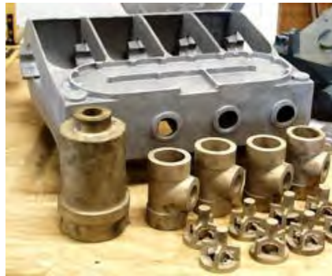
Figure 1: Engine castings for a replica of the Wright Brothers 1903 flyers engine showing engine block cast from Aluminum alloy and combustion chamber and ignition system components cast from Bronze.
