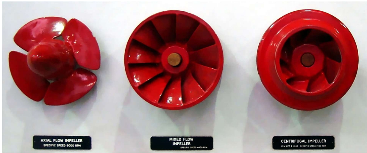
Figure 1: Example impellers for the three main impeller types for rotodynamic pumps. Source: commons.wikimedia.org/wiki/File:Pump_Impellers-1.jpg CC BY-SA 3.0
