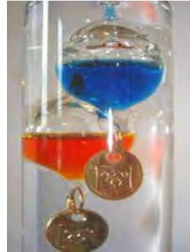
Figure No. 1 – Galileo Thermometer (Image Source: Wikipedia)
