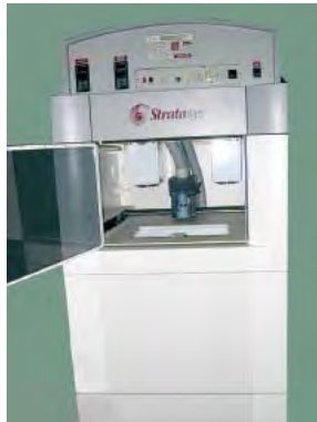
Figure 4. A picture of the 3D Modeler, the first commercial FDM 3-D printer developed by Stratasys.
