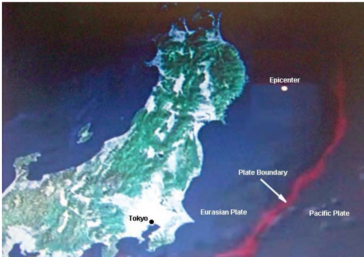
Figure 3: Location of the earthquake epicenter in relation to the mainland of Japan. The earthquake occurred as a result of an abrupt displacement between the Eurasian and Pacific Plates along their common boundary.
