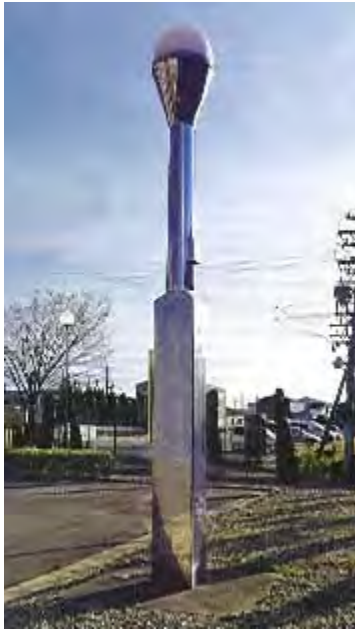
Figure 2: One of Japan's permanent GPS receivers used for monitoring earth movements.
