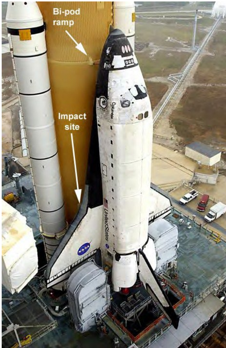
Figure 1 - The left bipod foam ramp which damaged the wing
