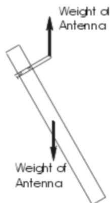
Figure 2: Model Riggers Should Have Used: Free Body Diagram of Lifting Bar and Analysis of Riggers' Solution
