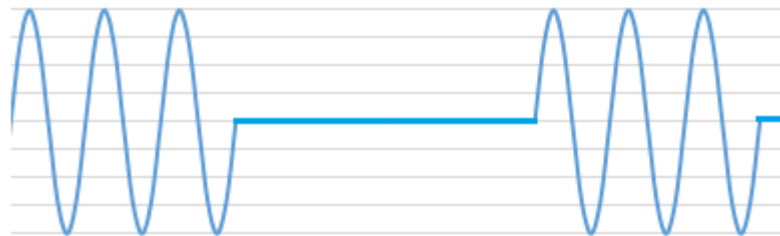
(C) Transmitted On-Off Keyed CW Signal
