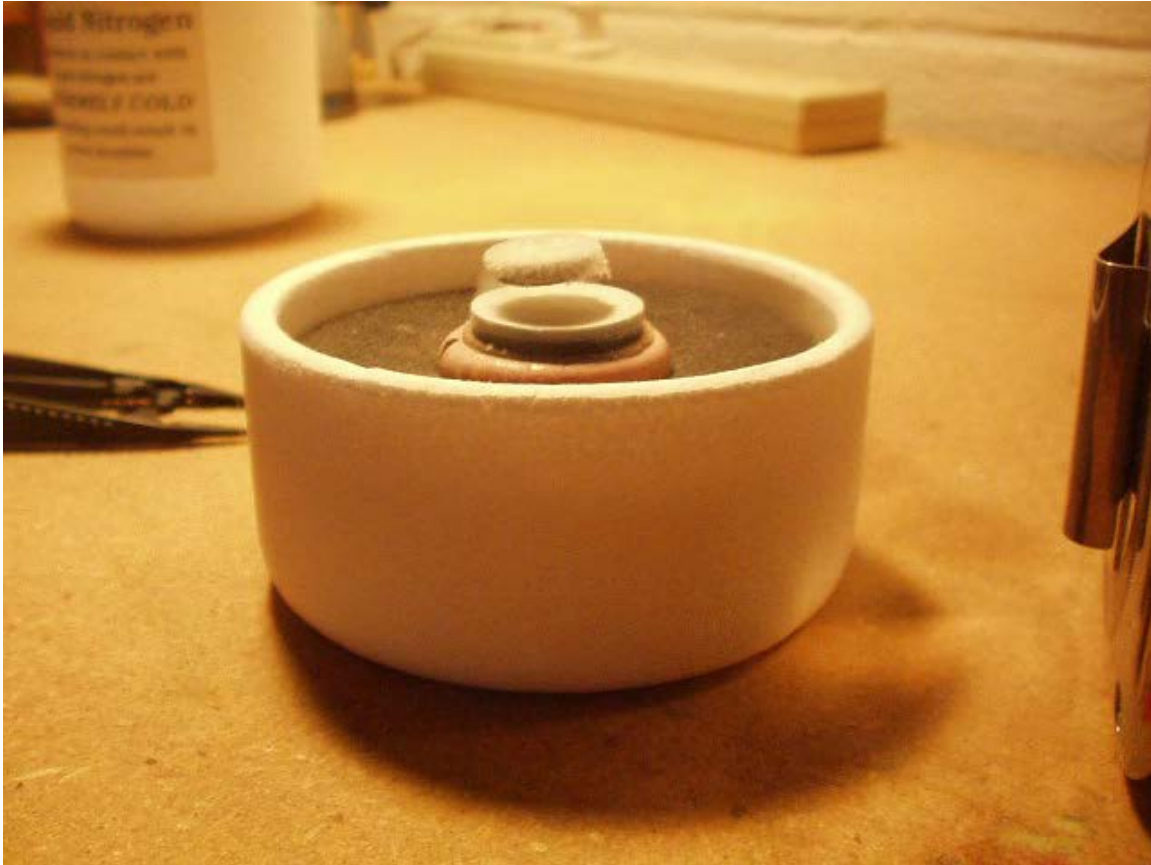
Figure 2. Neodymium-iron-boron magnet floating about .25" above a LN2 cooled yttrium-barium-copper-oxide superconductor. When I poured about a quarter of a cup of LN2 into the Styrofoam cup, the levitation effect lasted, amazingly, for almost 15 minutes before it needed a boost from another shot of LN2.
