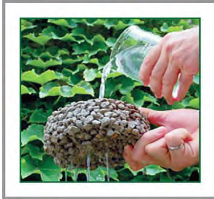
Figure 1. Pervious concrete; source - NRMCA
