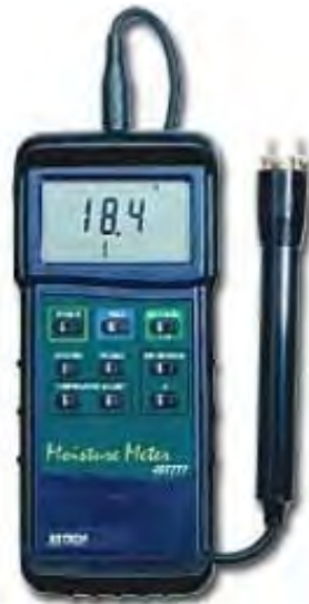
Figure No. 3 – Intrusive Style Moisture Meter
